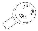
To operate the system on a lower amperage circuit, attach the female end of the 120 V / 15 A (NEMA 5-15P) plug adapter to the power supply's NEMA twist lock-style plug.
