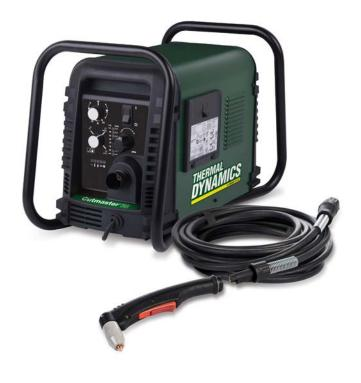
The Cutmaster 58 is the most powerful 1/2 in. (12 mm) machine on the market today. This unit cuts through mild, stainless, or aluminum up to 1-1/8 in. (30 mm) thick. The Cutmaster 58 combines power with the well-known performance and features of the industry-leading 1Torch®.
