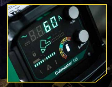
**Consumables end-of-life indicator** – Cutmaster 60i's end-of-life indicator monitors the remaining life of the consumable parts and alerts you when it's time to replace, maintaining optimal performance and cut quality.
