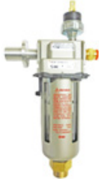
Old air filter assembly (with metal guarded filter bowl)
