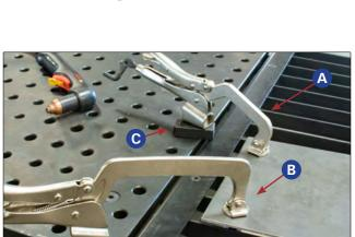
Insert the Inserta Pliers into the 5/8" holes on the Rhino Cart<sup>®</sup> Tabletop.
