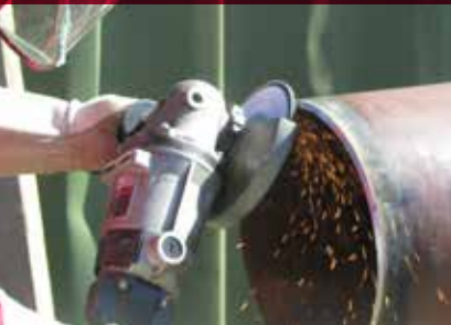
Edge chamfering a section of pipe with a Tiger Aluminum Back flap disc.
