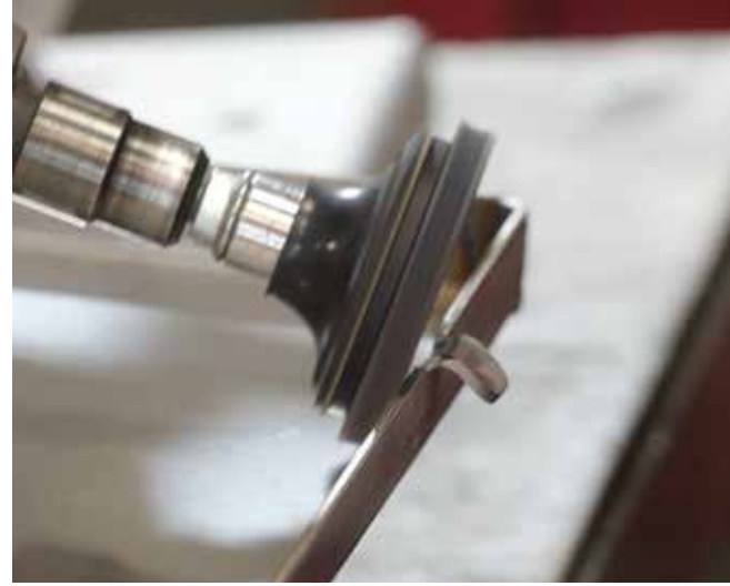
Edge chamfering a fabricated stainless steel component.
