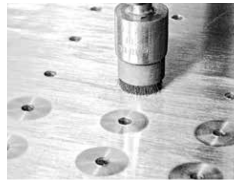
Cleaning around rivet holes with a pilot bonding brush.
