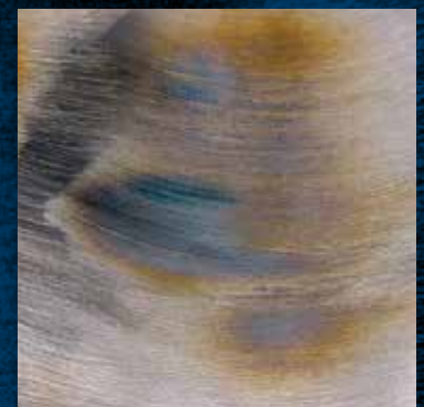
Typical heat discoloration on stainless steel.
