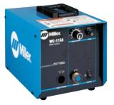
WC-115A Weld Control #137 546 Without contactor #137 546-01-1 With contactor This control operates on 115 VAC, and is designed primarily for CC DC power sources. It can also be used with CV power sources or DC engine drives supplying 115 VAC. When used with a CC source, the
