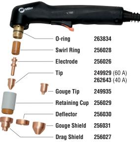
Note: Replacing drag shield with deflector offers improved arc visibility while maintaining 1/16-inch standoff. For gouging, replace the tip and drag shield with gouge tip and gouge shield. The rest of the XT60 consumables are common.
