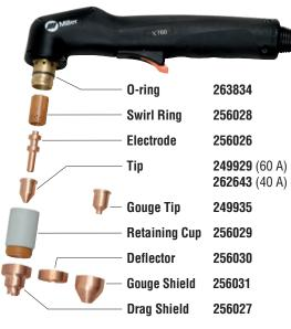
Note: Replacing drag shield with deflector offers improved arc visibility while maintaining 1/16-inch standoff. For gouging, replace the tip and drag shield with gouge tip and gouge shield. The rest of the XT60 consumables are common.
